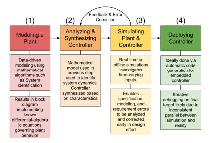
Fig 1. Summary of model-based design flow
